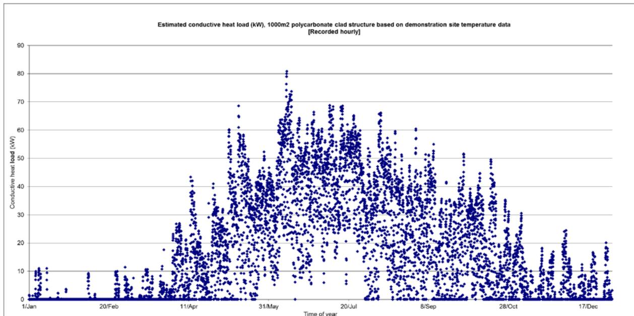
Figure 7 Conductive heat loss hourly averaged for a calendar year
