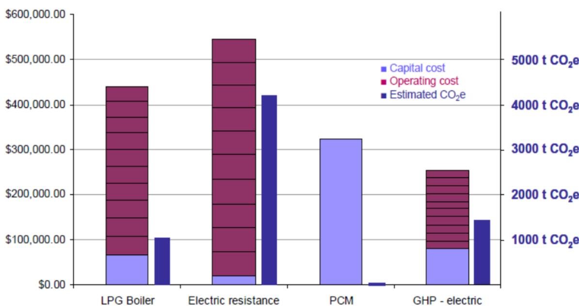
Figure 9 Cumulative cost analysis over 10 years of alternate energy options
