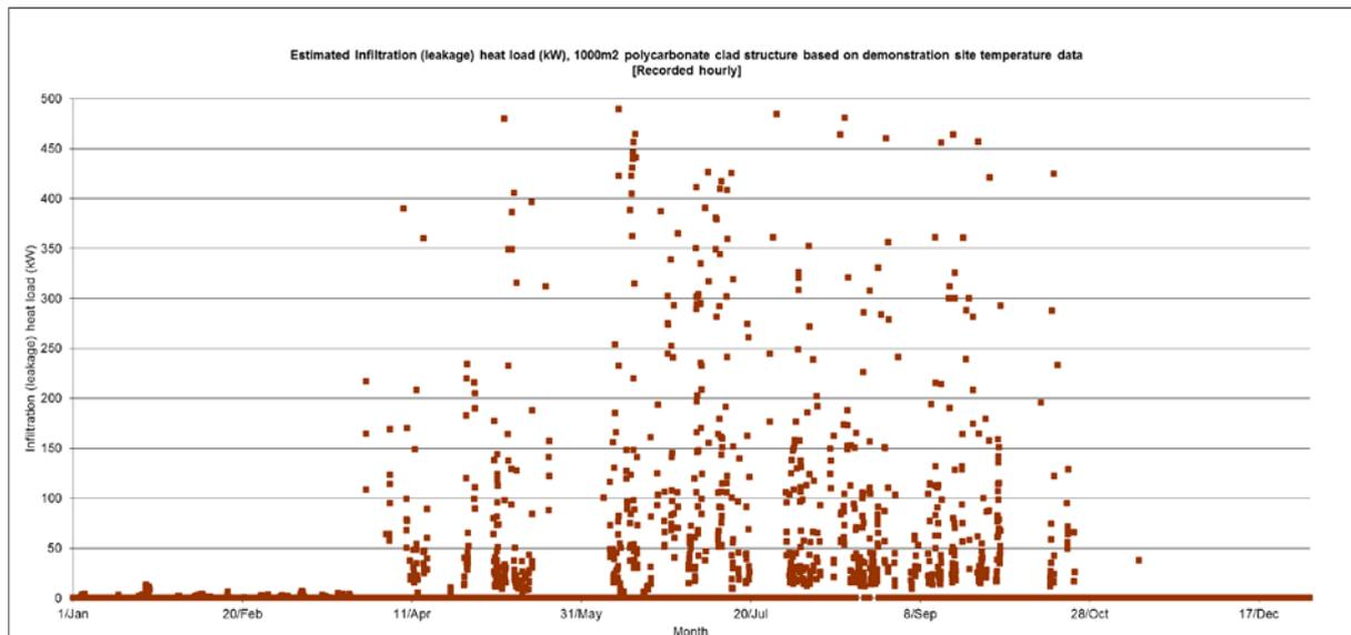
Figure 8 Infiltration heat loss hourly averaged over a calendar year
