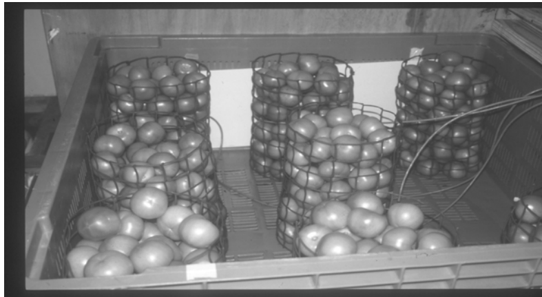
Figure 3. Mesh cylinders containing tomato fruit under test, positioned inside bin prior to filling the remaining space with low value filler fruit.
